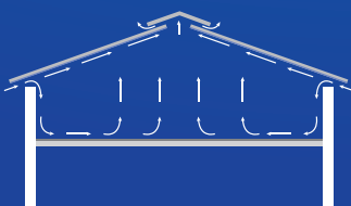
Adequate ventilation in an insulated building with air supply on the sides and air outlet through the roof ridge.
